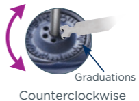
Figure 6 Adjust PIPETMAN® L fixed volume setting to compensate for a specific density or viscosity
