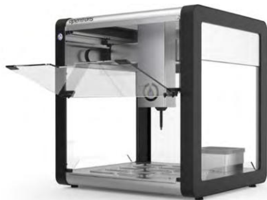
Figure 1: The Opentrons OT-2 is equipped with the Opentrons Magnetic Module and Opentrons GEN2 Pipettes for NGS clean-up. The Magnetic Module uses high-strength magnetic bars that can be engaged to magnetize magnetic beads, and disengaged to allow magnetic beads to remain in solution.
